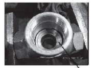
Clean and inspect seat sealing surface in body.
